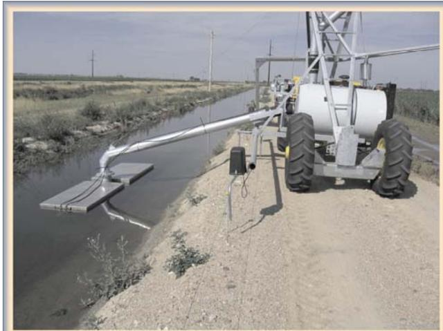
Fig. 4 - Water Supply for Linear Sprinkler
